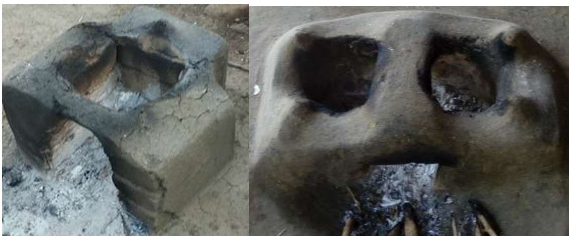
Figure 15: Image of C-type and inline stoves
